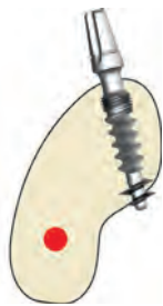
Bicortical anchorage of a KOS® Plus implant in the atrophied distal mandible.
